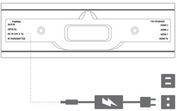
2. Plug the subwoofer's power cord into an active, unswitched AC outlet.
