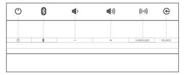
**Power Button**: The Power button turns the SABRE SB35 ON/OFF. When the SABRE SB35 is in Standby mode (Power Indicator is amber), press this button to turn the SABRE SB35 system ON (Power Indicator turns white).
