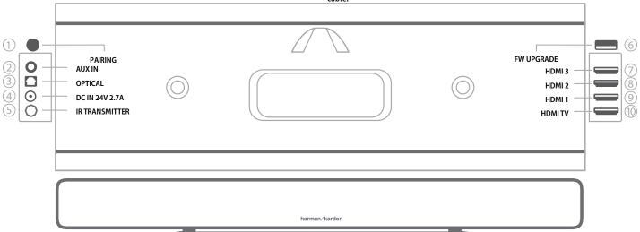
**Optical (digital optical audio in)**: If your TV, disc player or cable/satellite tuner has an optical digital output, use the included optical cable to connect it here.
