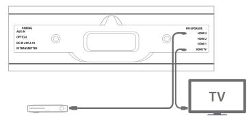
**HDMI In 1/2/3**: If any of your source devices have HDMI connectors, connect them to the soundbar's HDMI In 1/2/3 connectors for the best possible video and audio performance quality. Since the HDMI cable carries both digital video and digital audio signals, you do not have to make any additional audio connections for source devices you connect via HDMI connectors.
